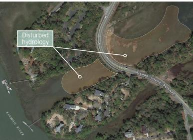
Left: Mingo Point was identified as a hot spot of concern due to erosion occuring along the bank of the Kiawah River. While-erosion on the outside bank of a stream is natural, in this location it could eventually undercut the road and parking infrastructure, as it has at Beachwalker Park. As seen on previous pages, there are a suite of management techniques that could be used here, including Envirolok and other nature-based bank stabilization designs.
